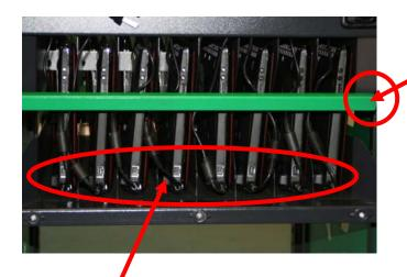
When transporting the laptops both the green bars, either side of the trolley should be in place and locked.
